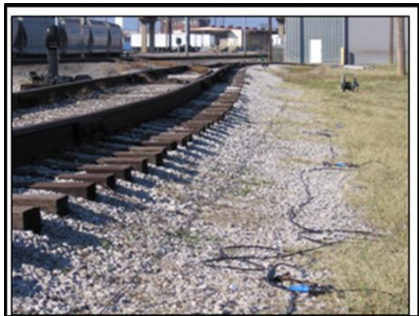
Figure 4. View along ReMi Line 1 showing 20-foot geophone spacings.
